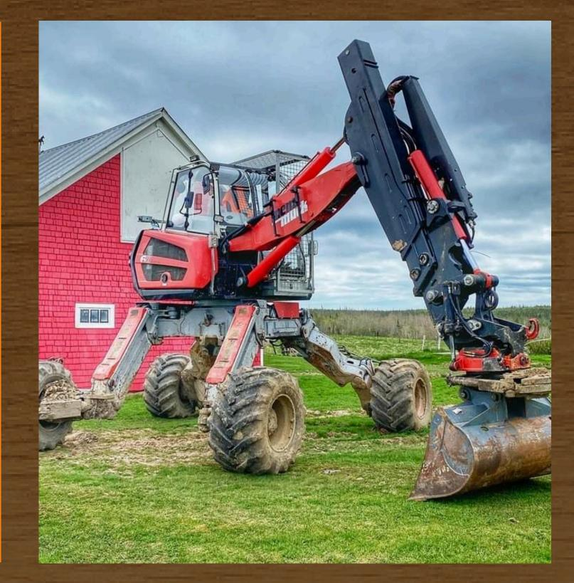
With its tilting body able to adapt to the subsoil, the powerful all-wheel drive and the possiblity to work on slopes up to 100% the range of use is almost inexhaustible, with boundaries nearly absent.
