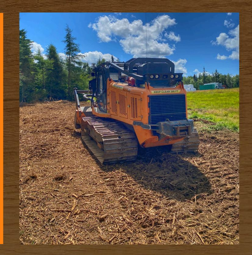
Its wide tracks allow for elevated power and low ground pressure making it the perfect machine for expanding and developing pastures, blueberry fields, riding trails, ATV trails, clearing lots for homes & more.
