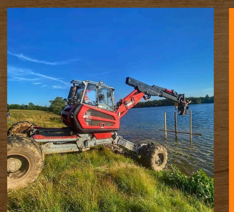
This is an extremely versatile European machine with 4 individually moveable legs. Various hydraulic cylinders enable the all-rounder to adapt its wheels and supports to any terrain. Allowing this machine to function at ease in difficult conditions.
