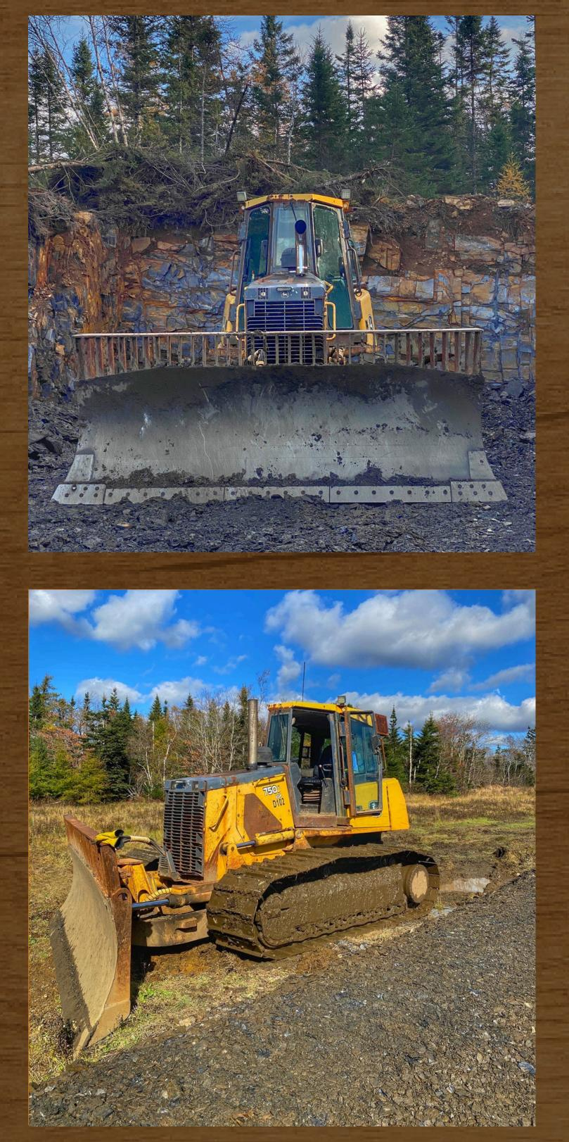
This Dozer is powerful and efficient, with its six way blade it is perfect for any landshaping, the wide tracks allow this machine to work even in swampy grounds with low ground pressure. Pushing earth, trees or rocks, building roads, or pulling vehicles
